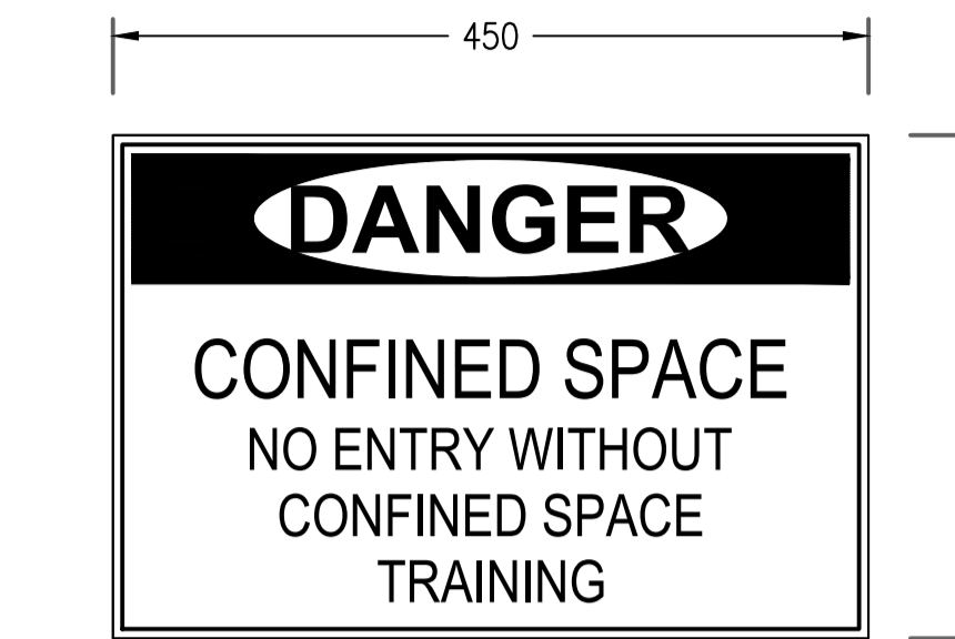
CONFINED SPACE SIGN DETAIL SCALE 1:20
